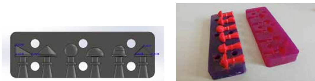
18. Joanna Rusin, spatial silicone elements - technical drawing of the mold and prototype cast of elements
